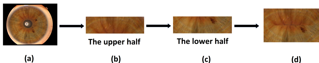
Figure 6 The proposed template generation for the Phoenix dataset. (A) Original image, (B) the upper half of iris, (C) the lower half of iris, (D) the final iris template.
